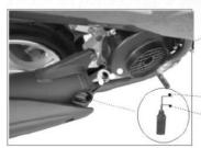
Level the motorcycle and fill in oil until the oil level is between the upper and lower markings.
