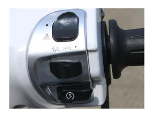
Push the electric startup button with your right thumb, and meanwhile turn the acceleration handgrip slightly with your right hand to add an appropriate amount of fuel.
