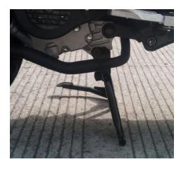
Then put up the main support. At the same time, the front wheel of the motorcycle must be towards an uphill direction so as to prevent the slipping of the motorcycle.
