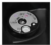
Start the ignition lock to check whether indicator lamps of instruments of the motorcycle work properly.
