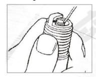
First, soak it with spark plug detergent or gasoline for about half an hour and then use a non-metal blade to remove the carbon deposit surrounding the spark plug, and finally clean the spark plug with gasoline.
