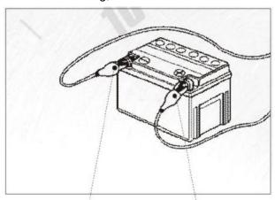
Check whether the connection of the accumulator cell is loose. It it is loose, tighten it.
