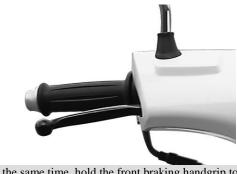
At the same time, hold the front braking handgrip to reduce the speed of the front wheel.
