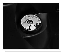
Turn the ignition lock switch to the position " to prevent the motorcycle from being stolen.
