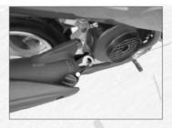
First, twist off the oil gauge and check whether the lubricating oil becomes black or deteriorated.
