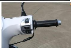
Hold the front braking handgrip, turn on the electric startup switch and perform electric startup.
