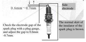
Take off the spark plug. If it is found that the color of the insulator skirt of the spark plug is brown, it indicates that the engine works properly, and there is nothing wrong with the spark plug.
