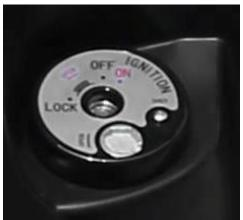
First, insert the key into the ignition switch lock, and turn it to the position "".
