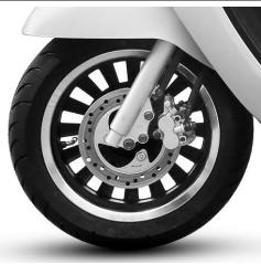
Check the air pressure of the tire and check whether the rim deforms. If any abnormality is found, it should be handled properly.
