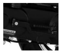
Step down the starting arm to its limit, and then reset the starting arm in time. The starting arm must be reset in time after the startup of the motorcycle.
