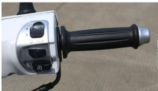
The accelerator handgrip should work smoothly. The idling clearance of the handgrip should range from 2mm to 6mm.
