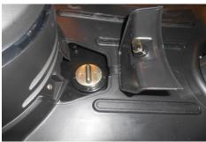
Seat cushion: Insert the ignition lock key into the seat cushion lock and turn it 90° clockwise to open the seat cushion.
