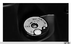
Turn the ignition lock key to the position "\overline{\times}" of the ignition system and stop the motorcycle.
