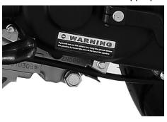
③The Engine Number is printed on the left lower part of the crankcase.
