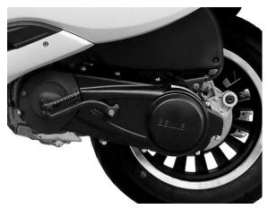
Take off the fastening screws of the air filter cover, and remove the air filter cover. Check whether there is too much dust on the sponge foam of the filter element. Take off the sponge foam.
