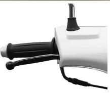
Hold the rear braking handgrip to reduce the speed of the rear wheel.
