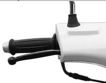
Turn the acceleration handgrip slightly with your right hand to add an appropriate amount of fuel to start up the motorcycle. The motorcycle can be run only after it is pre-heated.
