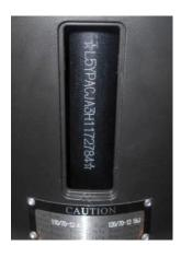
① The motorcycle Vehicle Identification Number (VIN) is printed on the vertical tube of the frame.
