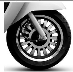
Check the tread wear depth of the tire casing and whether there is any crack. If any abnormality is founded, the tire casing should be replaced immediately.
