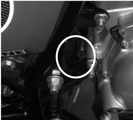
Rear brake light switch is located at the right side of chassis. Adjust rear brake light switch as follows: Lift or lower the switch, so that, when the brake pedal is pressed, the lamp is lit before feeling a pressure.
