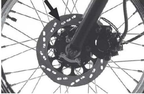
The essential of checking the front wheel brake lining is to see if the lining is worn to the limit mark. If wearing exceeds the mark, the brake lining shall be replaced with a new one.
