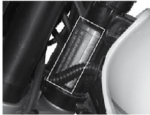
Chassis number (or VIN code) and engine number is necessary for registration of your motorcycle. Such numbers are needed with order components or service, to allow the distributor to provide you with better service.
